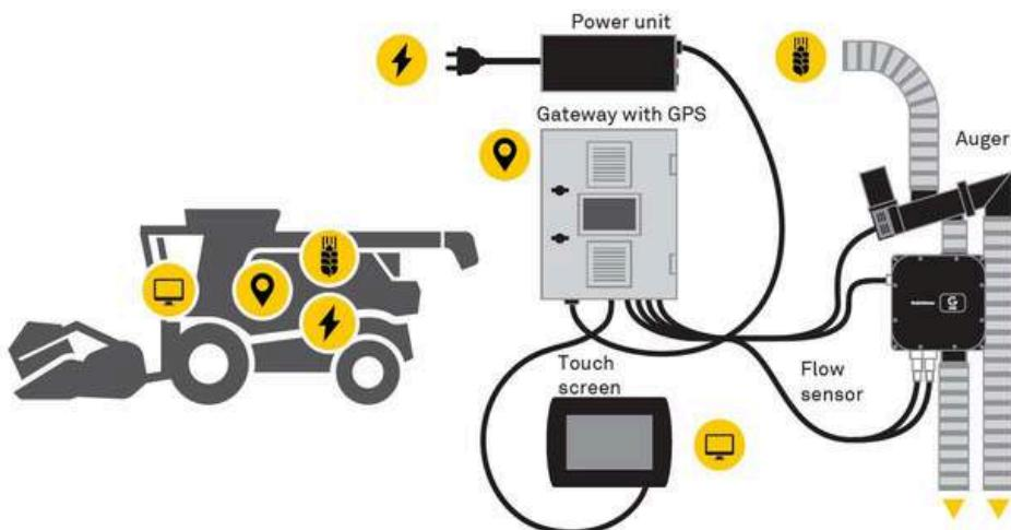
Via a grain entry and exit pipe system, grain is flowing through the GrainSense Flow® sensor, where real-time analysis is performed. The measurement data is sent to the GrainSense Cloud, enabling the farmer to monitor the measured results in real-time and to make better decisions. The user also gains access to heatmap visualizations generated from measurement data combined with location information.
